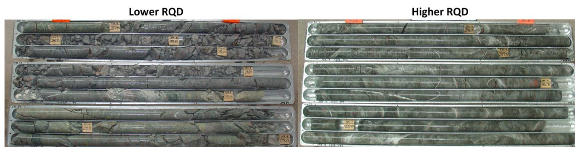
Figure 5 – Examples of core RQD
