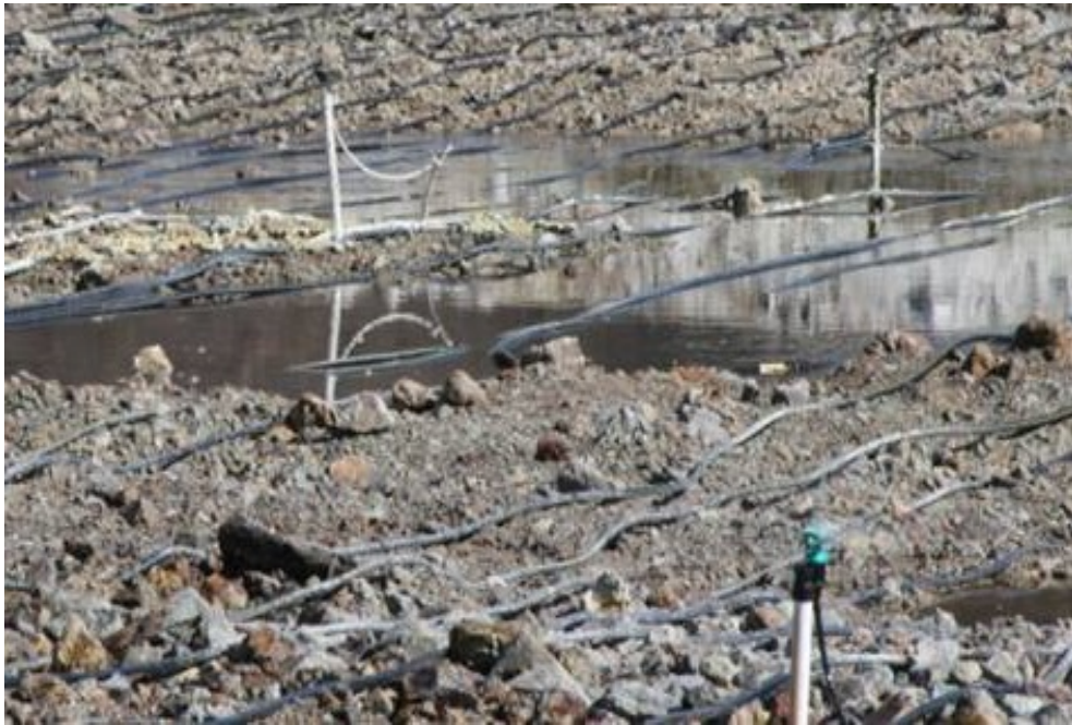
Figure 1: Photo of excess sprinkler and drip emitter solution application causing surface ponding
